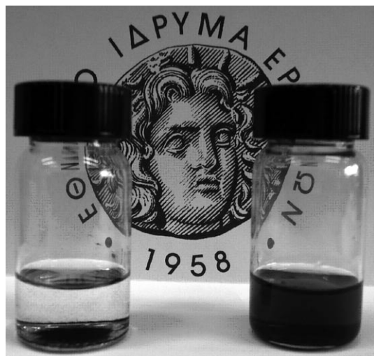
Figure 1. Photographical proof of soluble CNHs covalently functionalized with living polystyrene- b -polyisoprene block copolymer (right, after standing for one month) as compared with the insoluble CNHs (left) from the blank experiment, after standing for one month.
